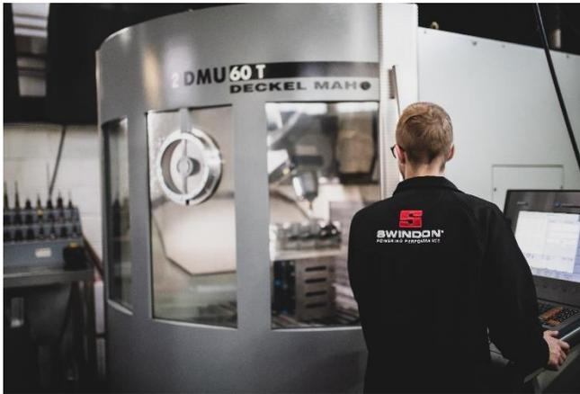
The DMG 5-axis machining centre has been busy on cylinder head manufacturing for a wide range of engine projects from iconic historical race engines through to the latest engine developments for the 2021 BTCC TOCA engine programme.
